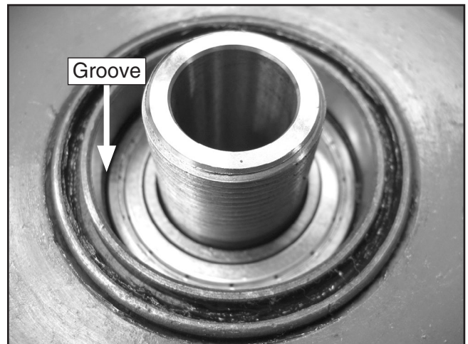
Figure 11. Installing new spindle.
